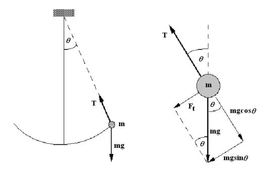
Figure 8.1: Force diagram of a pendulum
